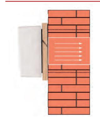
Many cellars already have core drillings, but not always with the required diameter for the fans. In order to use these core drillings also for the fans type 100-150 as well as 100-230, there is now an adapter plate available, which is mounted centrically on the existing hole.
